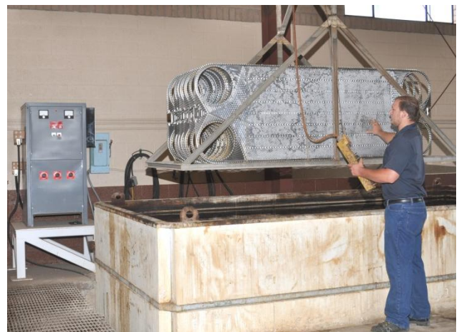
Acid etching-caustic chemical immersion
