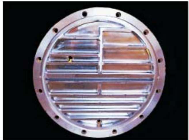
26-pass waterbox for pharmaceutical application
